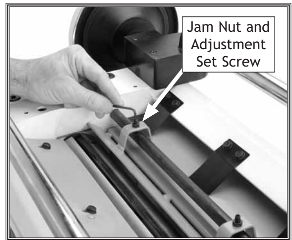
Figure 41. Chip breaker height adjustment.
